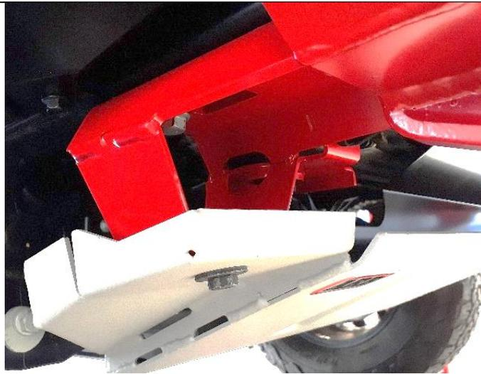
17. Fasten bullbar stone shield & either OEM Underpanel or UVP to recovery point cage nut using M10x30 flange bolts included in bullbar bag kit.
